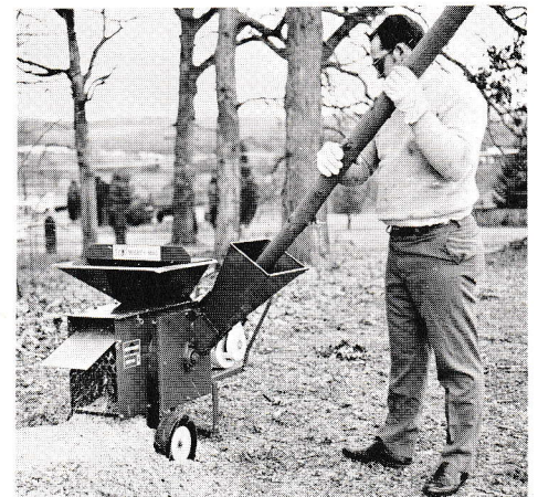
Model 12-P log chipper 6 hp. Will grind 3" thick logs. Also available as an attachment to 2 wheel Gravelys- Model 12-GC.
