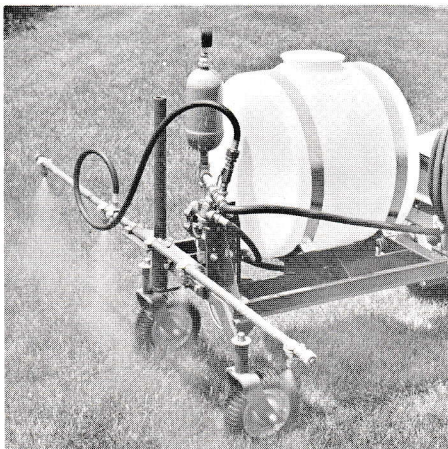
Model GC-TS shown with optional 4 nozzle spray boom and optional pulsation dampner.
